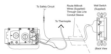
*Note:* If any of the original wire as supplied must be replaced, use 18 AWG TYPE CL2 (UL) 105 C (25 ft. length MAXIMUM) or equivalent.
